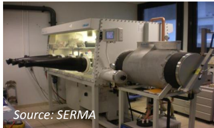
Glove box – Argon saturated For cell disassembly
