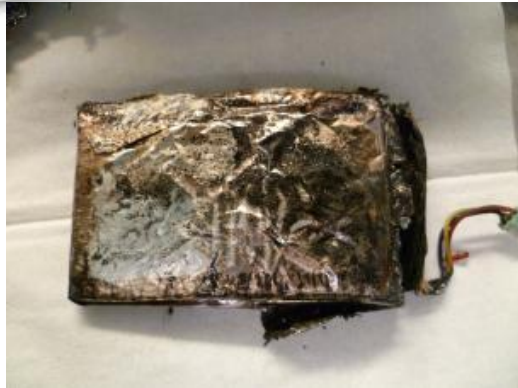
Battery after thermal runaway As received
