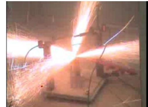
Degassing and Fire with 18650 Cells after Abuse Tests (source: es116_cunningham_2012)
