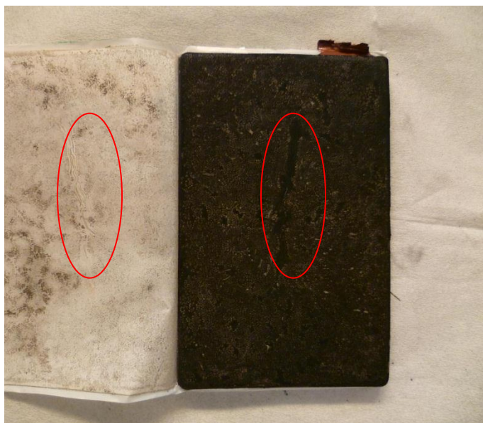
Cracks in anode layer due to a folded separator.
