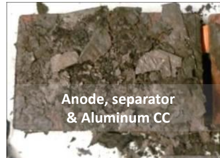
Micro short circuits localized
