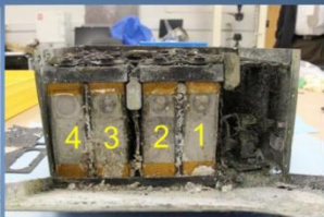
Moderate thermal damage
