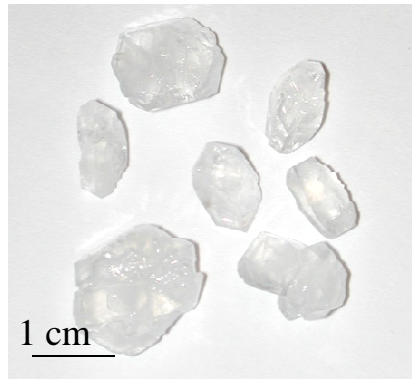
[\text{Ti}_8\text{O}_{12}(\text{H}_2\text{O})_{24}]\text{Cl}_8 \cdot \text{HCl} \cdot 7\text{H}_2\text{O} Crystals (1)
