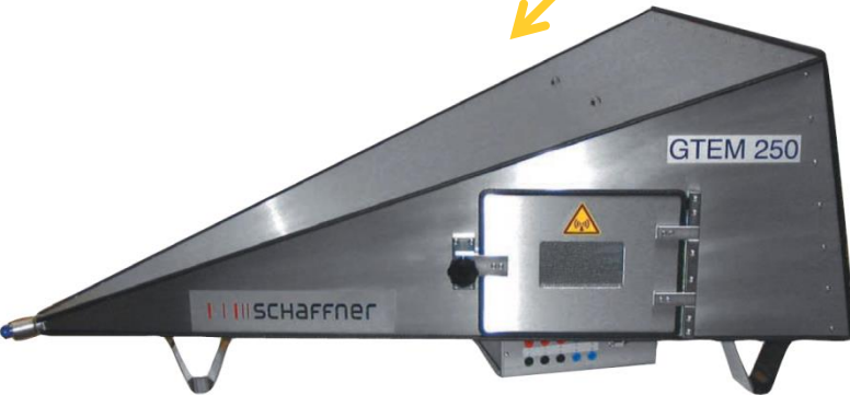
The Gigahertz Transverse Electromagnetic Mode "GTEM" cell
